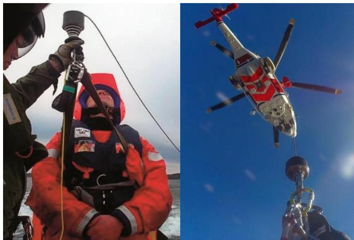
The helicopter may start by sending down a tag line (trail line). When the tag line has touched the deck, hold on to it but do not anchor it. The helicopter tag line is used to guide the surface swimmer or a stretcher when hoisted from/to the helicopter. With the tag line, you can help the rescue swimmer to reach the deck safely. Once the rescue swimmer is on board, he/she will give you further instructions. Do not question the instructions given by the rescue swimmer.
