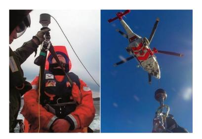
The helicopter may start by sending down a tag line (trail line). When the tag line has touched the deck, hold on to it but <u>do not</u> anchor it. The helicopter tag line is used to guide the surface swimmer or a stretcher when hoisted from/to the helicopter. With the tag line, you can help the rescue swimmer to reach the deck safely. Once the rescue swimmer is on board, he/she will give you further instructions. Do not question the instructions given by the rescue swimmer.
