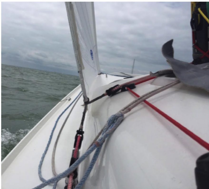
Jib clew shown In-hauled to about 1" from touching cabin house.
