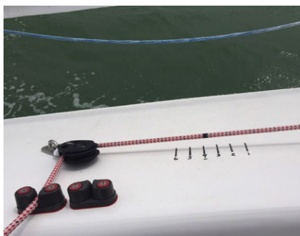
Jib sheet and deck reference marks help accurately repeat trim settings
