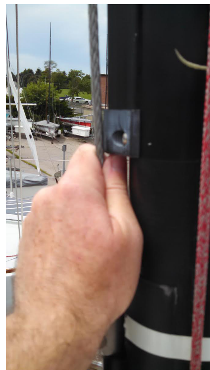
Hold main halyard to bottom of mast track to measure pre-bend
